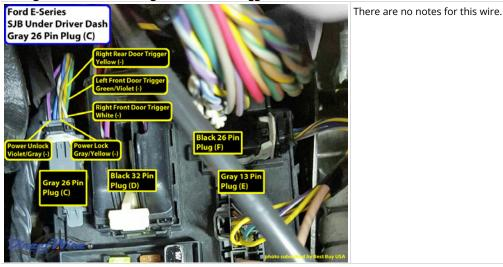
Wiring Photo and Notes: Right Rear Door Trigger
